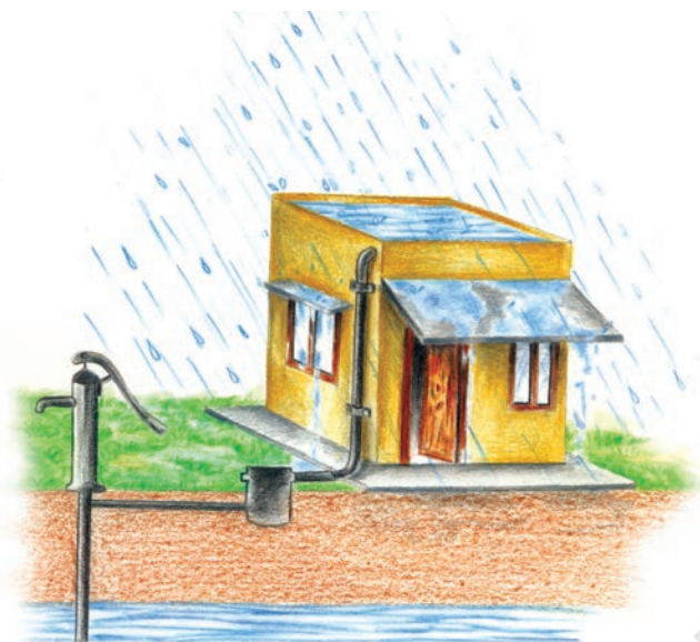
(a) Recharge through Hand Pump
